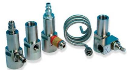
The sampling cells (from the left) DMT242SC2, DMT242SC and DSC74 can be used to connect the DM70 to sample gas flow. The DSC74B (right) is a two-pressure sampling cell that can be used for measurements in either pressurized or ambient pressure. The cooling/venting coil is included in the DSC74C sample cell, but is an option for all sampling cells.
