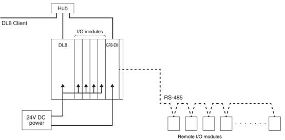
Note: It is not available to supply the power via DL8. Supply the power with the connector for power supply.
