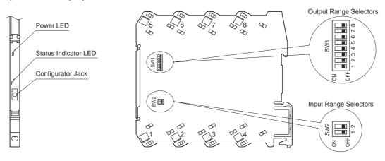
The DIP switch setting is required to select input and output types before setting a precise range using PC Configurator Software (model: M6CFG).
