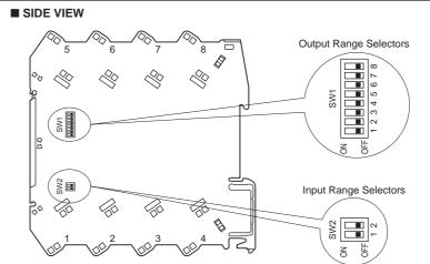
The DIP switch setting is required to select input and output types before setting a precise range using PC Configurator Software (model: M6CFG).
