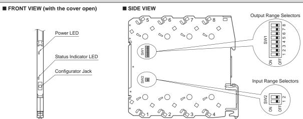
The DIP switch setting is required to select input and output types before setting a precise range using PC Configurator Software (model: M6CFG).
