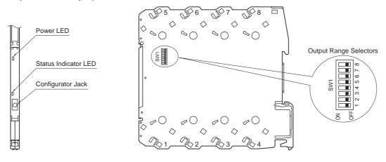
The DIP switch setting is required to select output types before setting a precise output range using PC Configurator Software (model: M6CFG).
